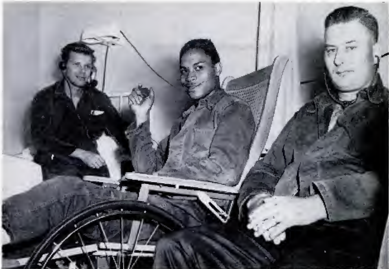
Listening devices can be provided to meet any patient's particular need. Bed patient wears conventional headset and man in center holds a plastic pillow speaker. Stethoscope headset, right, has special volume control
